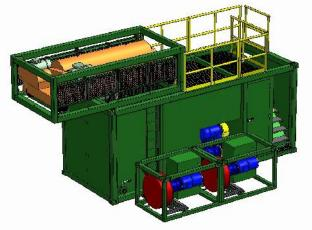
The centrifuge and its motors are mounted on a heavy-duty hollow section steel frame measuring  $4000 \times 1800 \times 1190$  mm high. The inverters, electrical controls, touch screen PLC, inverter controlled discharge pump and centrate collection tank are all housed in the Powerhouse Module, which also incorporates a staircase for access to the upper level.
